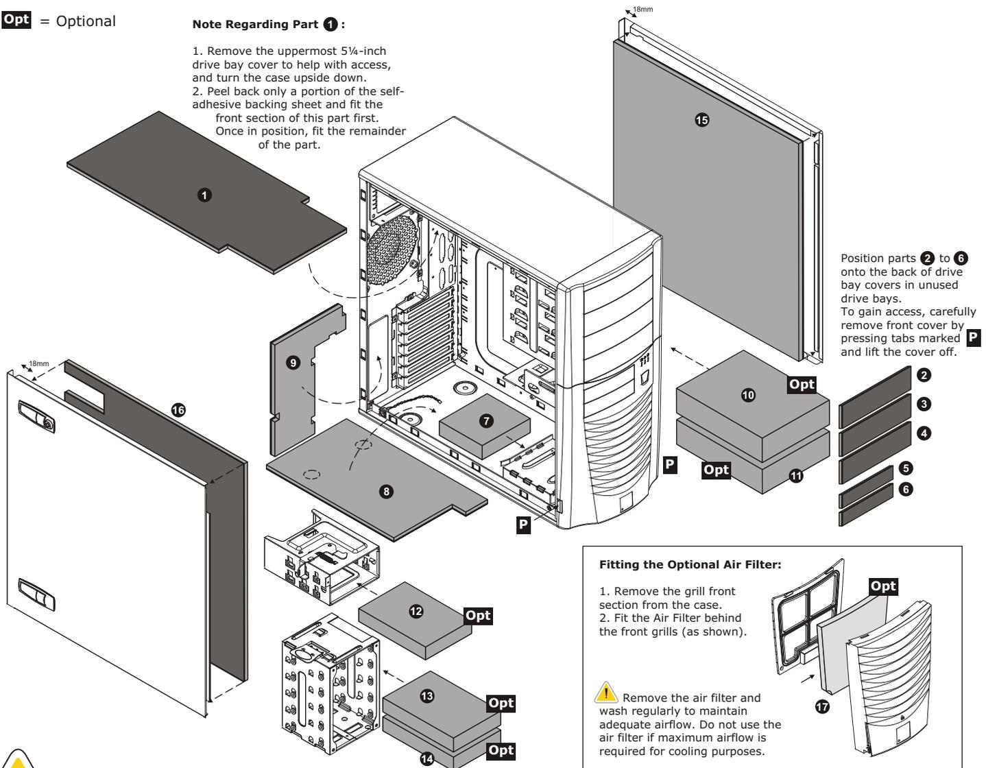
Position parts ② to ⑥ onto the back of drive bay covers in unused drive bays. To gain access, carefully remove front cover by pressing tabs marked **P** and lift the cover off.
